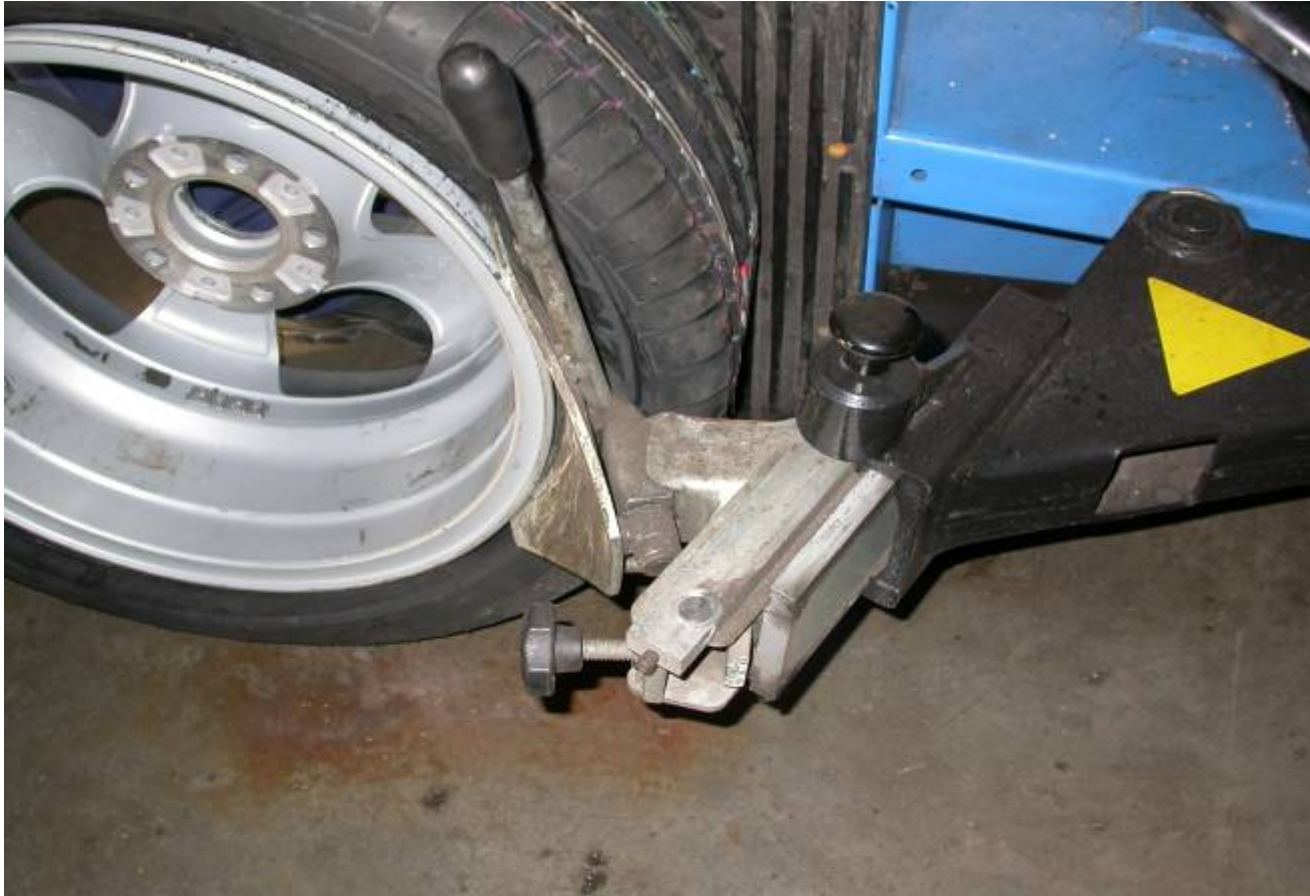
Bead breaker blade with travel limiter
